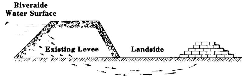
**NEVER completely stop the flow from a sand boil. This may cause the boil to "break out" in an adjacent area. ALWAYS control the boil to a point where it ceases to carry material and the water runs clear.**
