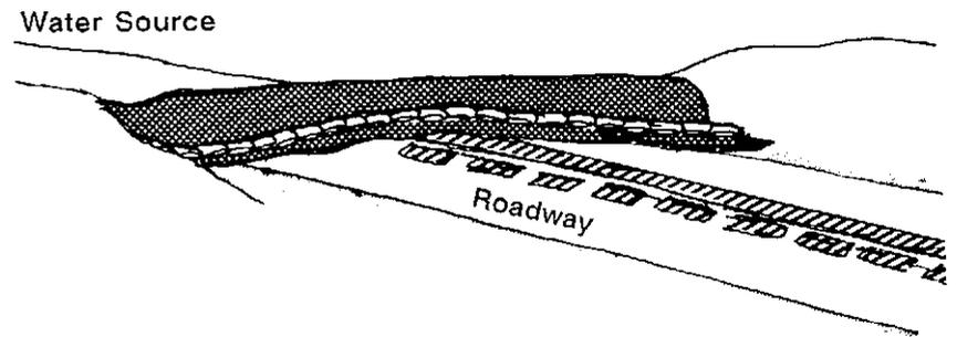
Place **fill material (sand, dirt, gravel, etc.)** on the visquine by hand labor or with equipment. Next, fold the visquine over the material from the waterside toward the landside. Finish by placing one solid row of sandbags on the edge of the visquine following procedures for sandbag construction in Figure 2. When used in overtopping of small earthen dams, a spillway must be constructed.
