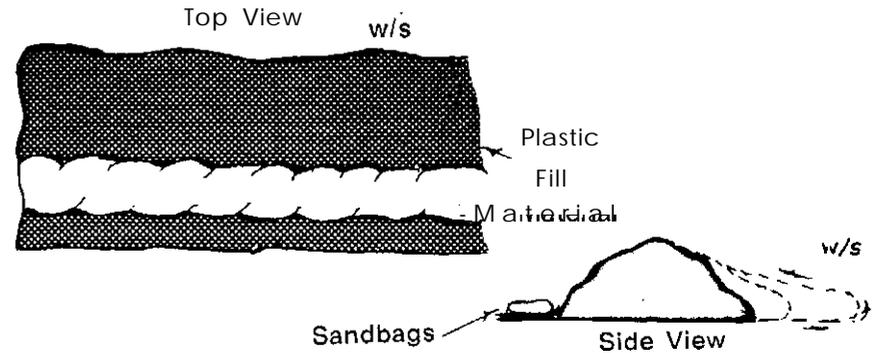
Lay plastic flat on area to be raised. Place fill material (dirt, sand, gravel, etc.) on plastic. Fold plastic back over fill material and lay a solid row of sandbags on lip of plastic.
